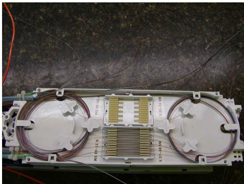
HEAT TUBE FUSION SPLICER HOLDERS SHALL BE MANUFACTURED BY TYCO ELECTRONICS PART # SMOUV-1120-01-US.
