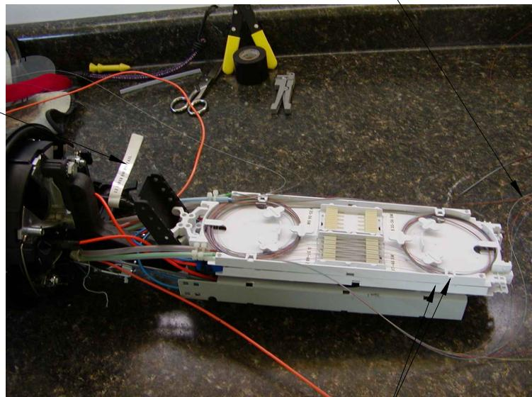
SEPARATE SPLICING TRAY FOR EVERY 2 TUBES OF FIBER INCLUDING NON-SPliced FIBER TUBES
