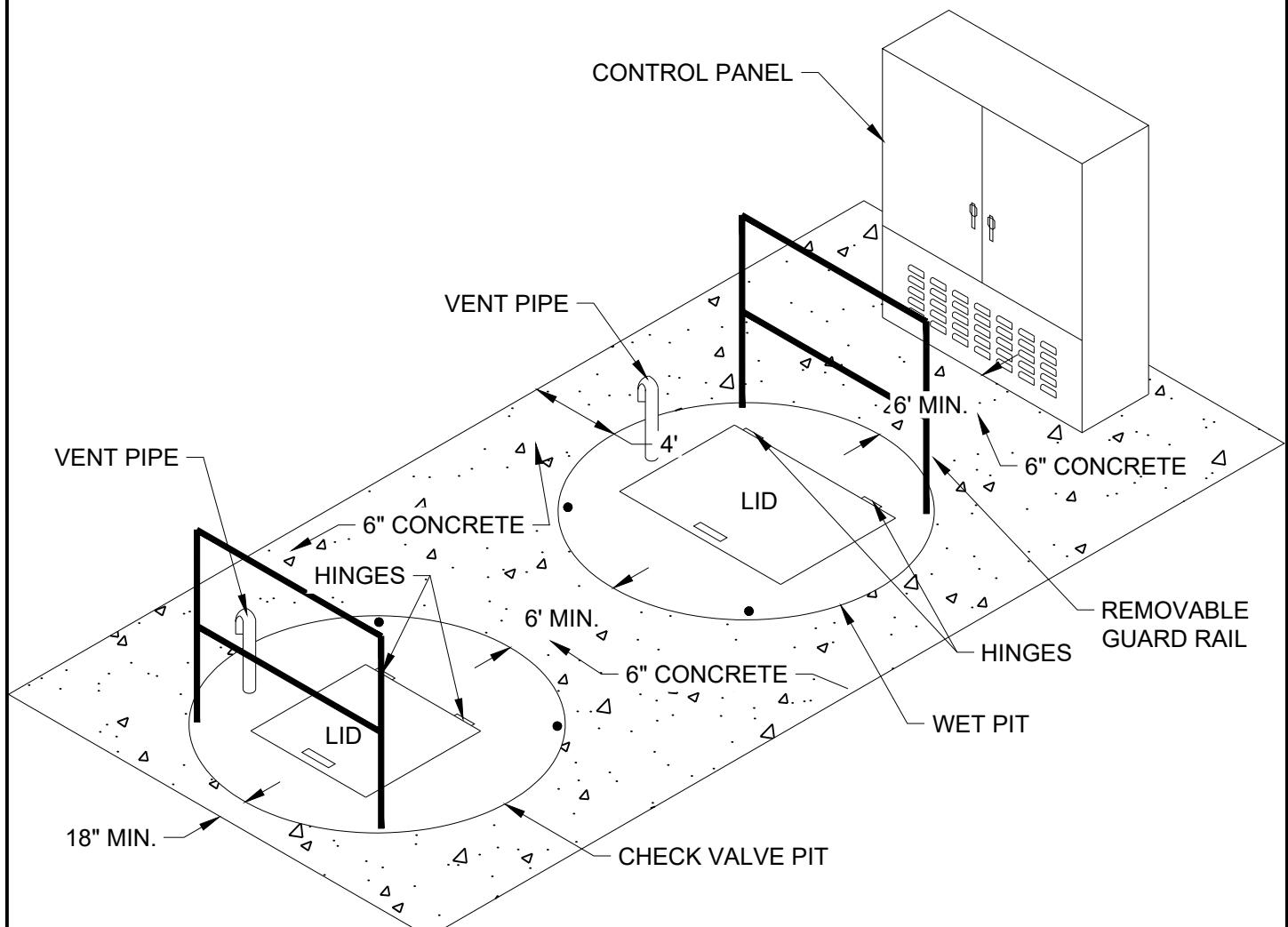
• - INDICATES HOLES IN CONCRETE COVER FOR GAURD RAIL RETENTION
